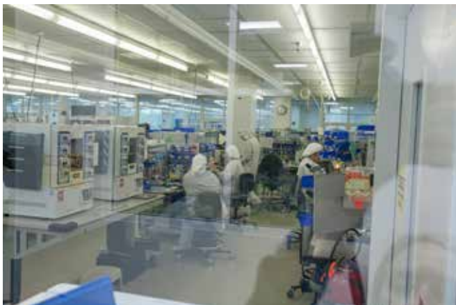
Photo 1: At KSE's Charlton, MA, facility, endoscopes and boroscopes are assembled from precision parts in several clean rooms by skilled technicians using microscopes and other tools.
